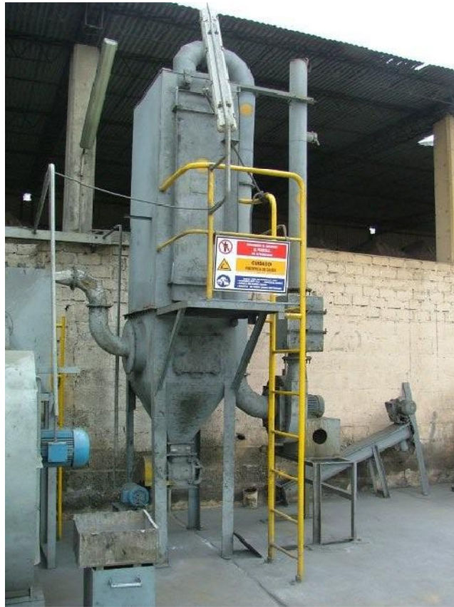
Figure 3 : The calcine collection system
