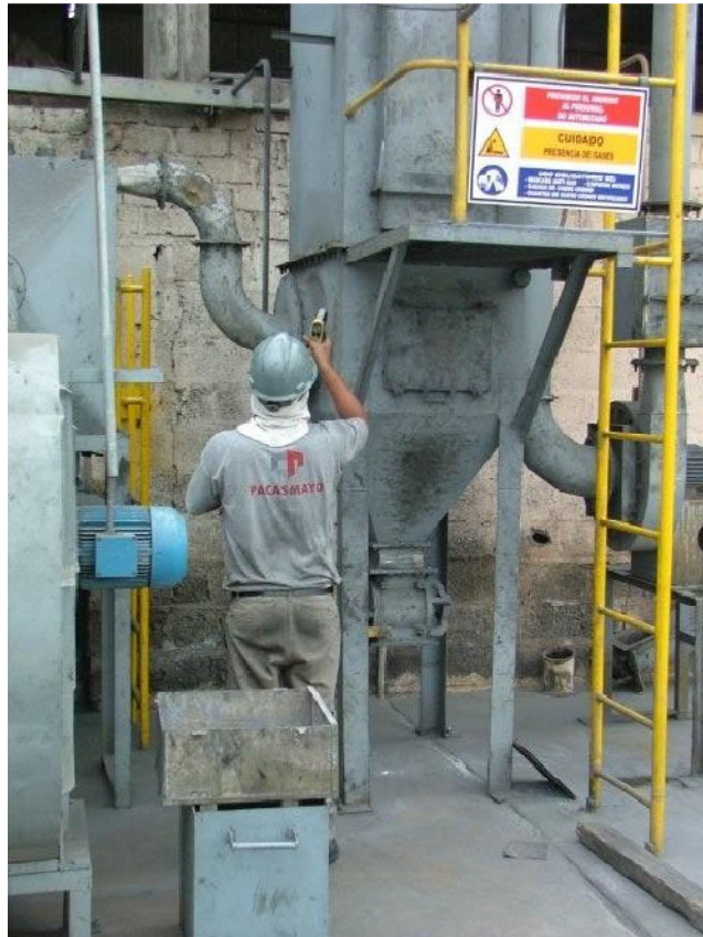
Figure 4 : Monitoring the temperature in the baghouse
