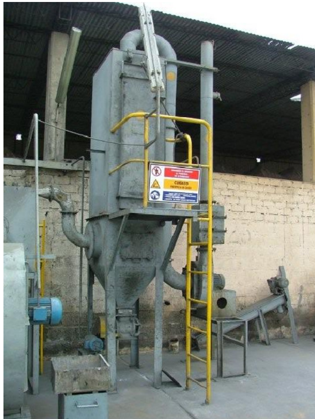
Figure 4 : The calcine collection system
